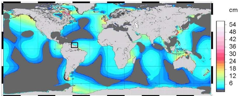
Figure 3. Predicted shifting of the mhwI under the 18.6 year nodal cycle for the next decade (adapted from the global map of tidal amplitude proposed by <sup>29</sup> by considering a modulation of signal of 3%). Grey areas correspond to locations of decrease or negligible rise. The black box (48W-62W-2N-12N) delimits the mud bank system of the Guyanas, South America.
