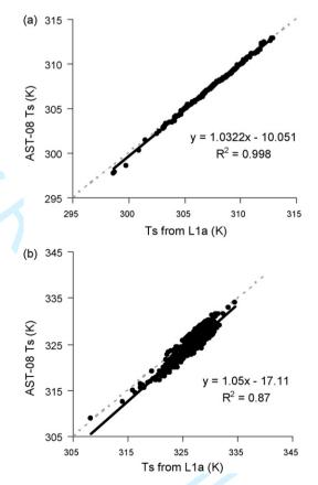
**Fig. 2.** Relationships obtained between land surface temperature (TES method) from L1a images and ASTER temperature standard product (AST-08) for (a) 12 March 2001 image and (b) 22 June 2001.
