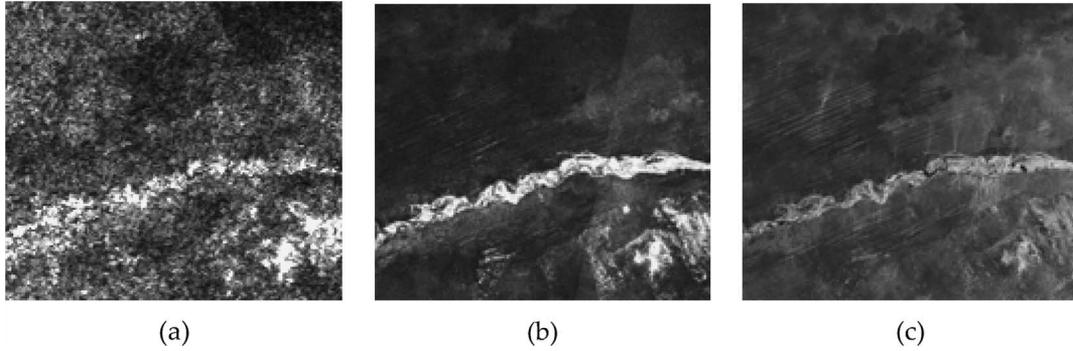
Fig. 3. Comparison of ASAR images of the same area ( $17.1^\circ$  N,  $1.6^\circ$  W) acquired in three different modes at VV polarization. (a) GM, (b) WS, and (c) IM modes. The size of the images is about  $75 \times 85$  km. The images were acquired during the dry season on February 24, 4, and 26, 2004 for the GM, WS, and IM modes, respectively.
