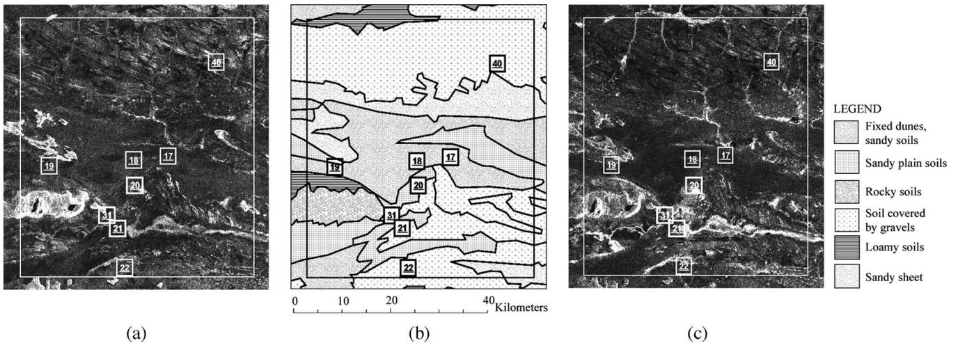
Fig. 4. (b) Comparison between the soil map and ASAR-WS images acquired at (a) VV polarization on October 10, 2005 and at (c) HH polarization on April 18, 2005.
