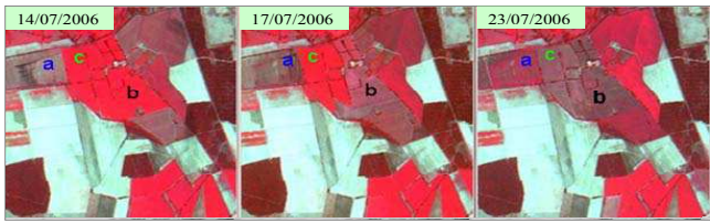
Fig. 2. Combination between 3 spectral bands ( G , R , NIR ) of FORMOSAT-2 images for 3 consecutive dates in July acquired over a small area (2×2 km) of the Crau region, showing the mowing of grasslands (in red): the “c” field was the last mowed.
