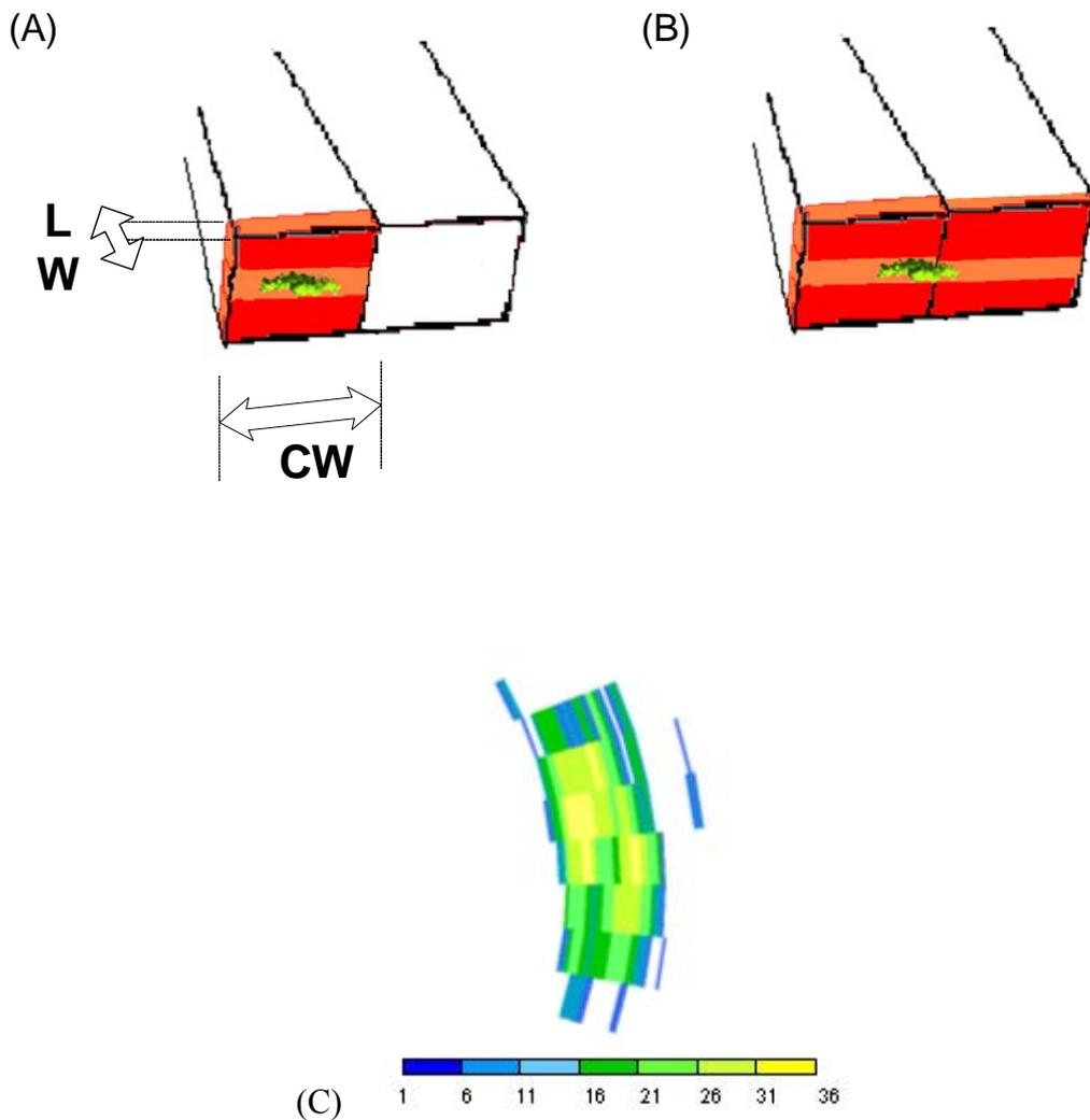
Fig. 3. Representation of the two sonar dimensions ‘Lw’ along and ‘Cw’ across the beam axis. (A) A school detected inside one of the 64 beams (in orange) that covers the whole beam volume detection area (in red). (B) The effect on the sonar echoes representation when a school crosses two beams: there is an extension of the Cw school dimension. (C) Zoom on a large school echo shape showing the heterogeneity of such biological structure (scale in acoustic intensity = 64 levels).
