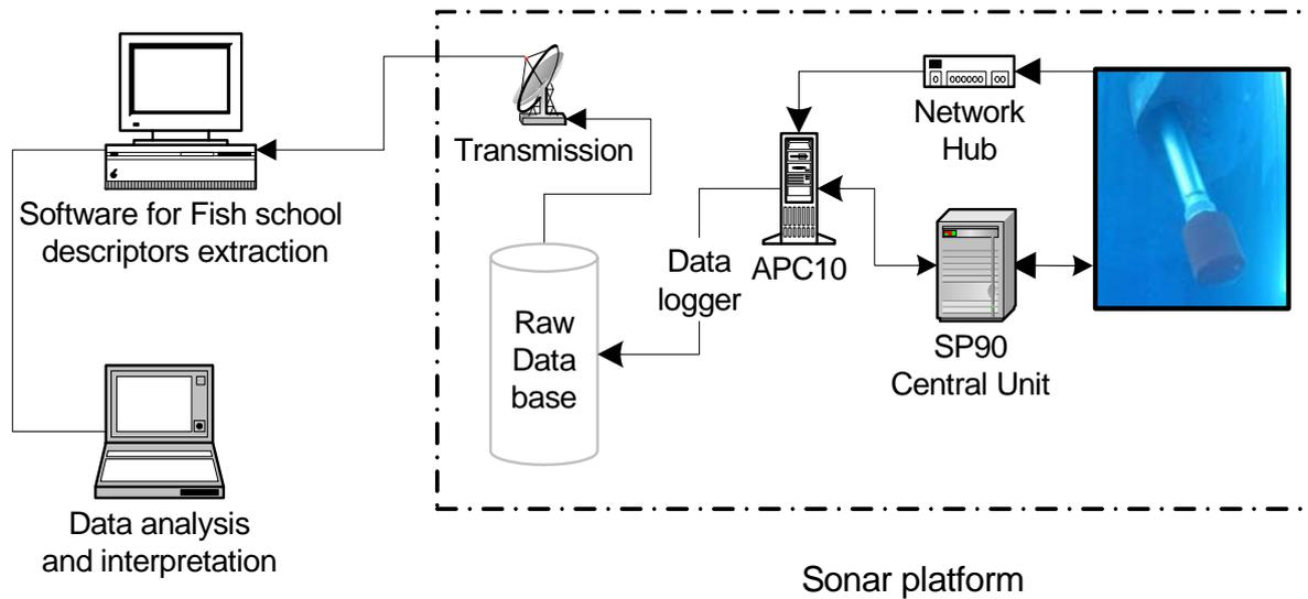
Fig. 1. Description of the tools and methods used to exploit (i.e. acquire, store/transmit, extract and analyze) the raw data delivered by the Simrad SP90 sonar. The dotted rectangle denotes the system components that are used during the surveys, and can be mounted either on a fixed or on a drifting platform.
