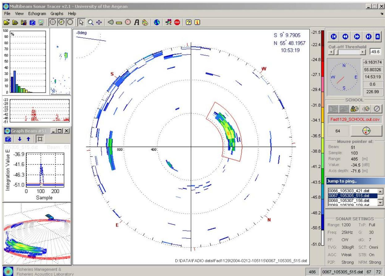
Fig. 2. Graphical user interface of the Multibeam Sonar Tracer software, illustrating the main panel, the multibeam echogram and statistical analysis results of fish schools around a Fish Aggregating Device (refer to Table 2 for school descriptors results).
