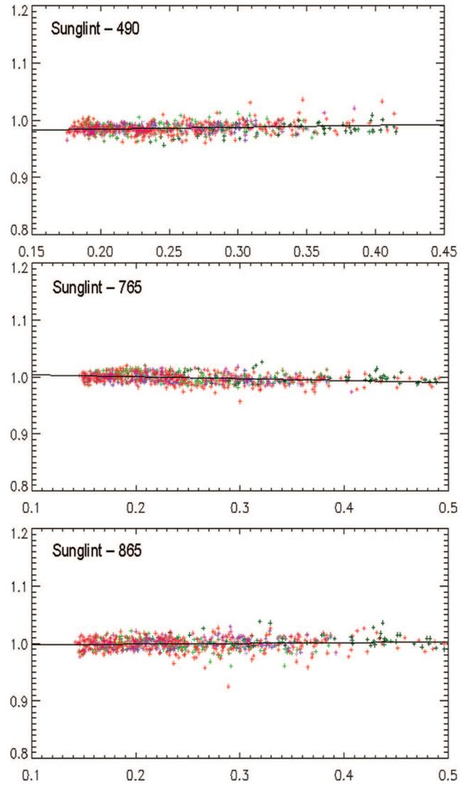
Fig. 5. (Color online) Interband calibration over sunglint. Measured to estimated radiance ratio  $\Delta A_k$  as a function of the estimated normalized radiance for spectral bands of 490 (top), 765 (middle), and 865 (bottom). Standard deviations are 0.88% for 490, 0.84% for 765, and 1.05% for 865 with  $N = 765$  points from March to May 2005.
