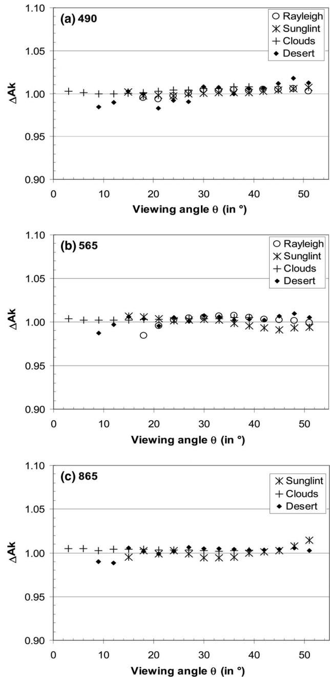
Fig. 13. Calibration results summarized as a function of the viewing angle for the 4 calibration methods. Measured to estimated radiance ratio  $\Delta A_k$  were averaged every 3 degrees for bands 490 [(a), top], 565 [(b), middle], and 865 [(c), bottom].
