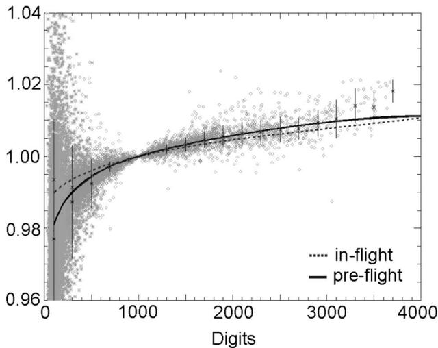
Fig. 12. Nonlinearity function as defined by Fougne *et al.* [9], derived from preflight characterization (plain line), and measured in-flight using SIT/LIT alternated acquisitions (diamonds). The in-flight estimated model (dashed line) is consistent with preflight model within 0.5%. All estimations have been normalized to 1.0 for digit 1000.
