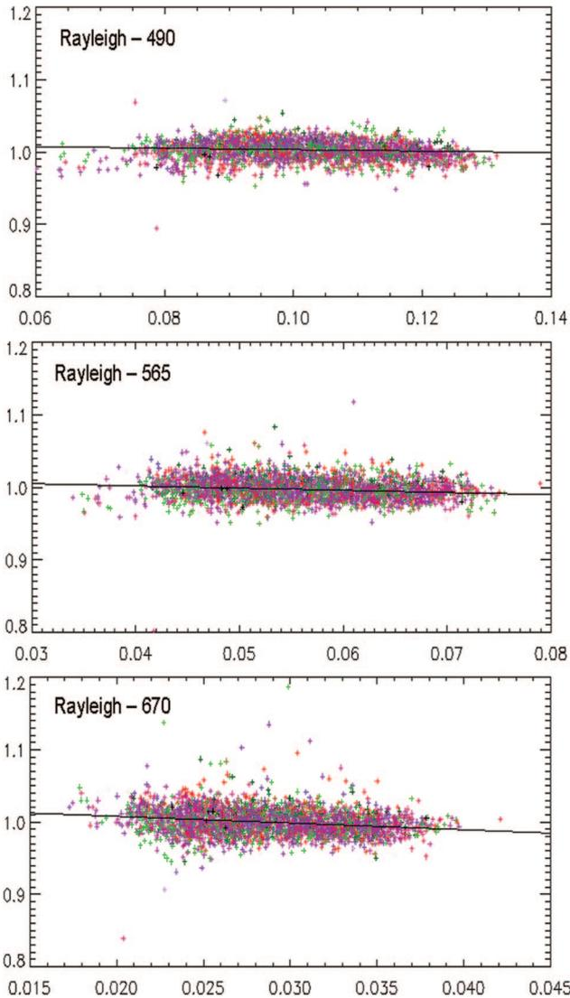
Fig. 4. (Color online) Calibration over Rayleigh scattering. Measured to estimated radiance ratio  $\Delta A_k$  as a function of the estimated normalized radiance for spectral bands of 490 (top), 565 (middle), and 670 (bottom). Standard deviations are 1.15% for 490, 1.38% for 565, and 2.29% for 670 with  $N = 4457$  points from March to May 2005.
