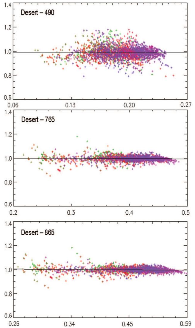
Fig. 7. (Color online) Calibration over desert sites. Measured to estimated radiance ratio  $\Delta A_k$  as a function of the estimated normalized radiance for spectral bands of 490 (top), 765 (middle), and 865 (bottom) using POLDER-2/ADEOS-2 as reference. Standard deviations are 4.61% for 490, 2.13% for 765, and 2.05% for 865 with  $N = 3941$  points from March 2005 to March 2006.
