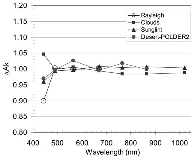
Fig. 8. Synthesis of PARASOL in-flight calibration results. Measured to estimated radiance ratio  $\Delta A_k$  for all PARASOL spectral bands and for calibration over Rayleigh scattering (circle), interband over sunglint (triangle), interband over clouds (square) and over desert sites using POLDER-2 as a reference (dot). Interband results (clouds and sunglint) reported here are renormalized to the mean of 490-565- 670 values to be comparable with results from the two other absolute methods.
