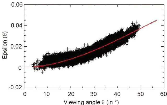
Fig. 11. (Color online) In-flight estimation of the polarization sensitivity of the instrument for the band 670,  $\epsilon(\theta)$ , based on measurements over clouds in specific geometries for which the observed target is unpolarized.
