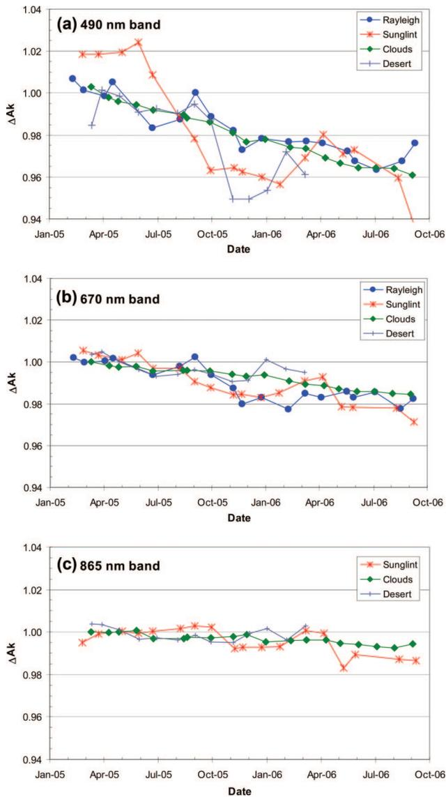
Fig. 9. (Color online) Temporal evolution of  $\Delta A_k$  from March 2005 to September 2006 for bands 490 (a), 670 (b), and 865 (c) as observed for various calibration methods. For one given spectral band and calibration method, the set of measurements is normalized to a reference value computed for 1 April 2005 using a linear regression on this set. For interband methods, the band 765 is used as reference and is supposed to be stable with time.
