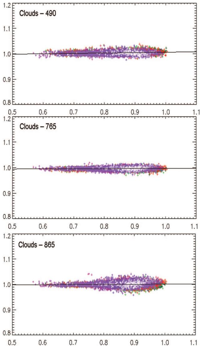
Fig. 6. (Color online) Interband calibration over clouds. Measured to estimated radiance ratio  $\Delta A_k$  as a function of the estimated normalized radiance for spectral bands of 490 (top), 765 (middle), and 865 (bottom). Standard deviations are 0.67% for 490, 0.54% for 765, and 0.87% for 865 with  $N = 10614$  points from March to May 2005.
