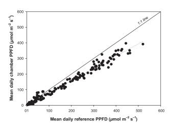
**Figure 7.** Relationship between the mean daily photosynthetic photon flux density (PPFD) reaching the fifth or sixth whorl from the top of reference and whole-tree chamber (ambient [CO<sub>2</sub>] only) trees for the period of 1 January–30 June 2002. The regression line was forced through the origin (y = 0.79x;  $r^2 = 0.98$ ; P < 0.001).
