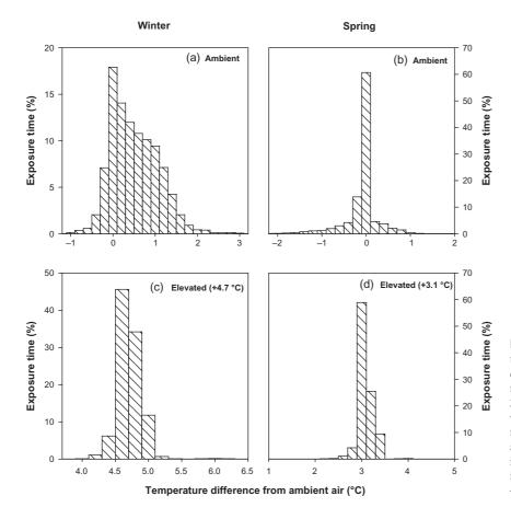
**Figure 5.** Frequency distributions of temperature in the ambient,  $T_A$  (a & b), and elevated,  $T_E$  (c & d), chambers for the measurement periods 14–28 February, and 3–17 May, 2002. Frequency distributions were calculated using temperature measurements from the six  $T_A$  chambers and the six  $T_E$  chambers measured at 42 min intervals. The target temperature elevations in February and May were +4.7 °C and +3.1 °C, respectively.
