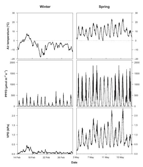
**Figure 3.** Flakaliden climate [air temperature, photosynthetic photon flux density (PPFD) and water vapour pressure deficit (VPD)] for 14 d in February and 14 d in May 2002. The data shown are measurements made at 3 min intervals. Air temperature was measured at a height of 2.5 m and PPFD was measured at 11 m.
