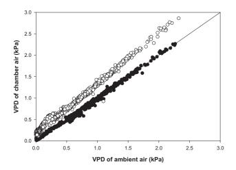
**Figure 6.** Water vapour pressure deficit (VPD) of an ambient temperature,  $T_A$ , chamber (filled symbols) and an elevated temperature,  $T_E$ , chamber (open symbols) by reference air VPD. Data from the time periods of 14–28 February and 3–17 May 2002 are pooled for each chamber.
