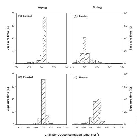
**Figure 4.** Frequency distributions of  $[CO_2]$  in the ambient,  $C_A$  (a & b), and elevated,  $C_E$  (c & d), chambers for the measurement periods 14–28 February and 3–17 May, 2002. Frequency distributions were calculated from the central IRGA measurements made on a 42 min cycle from the six  $C_A$  and six  $C_E$  whole-tree chambers, respectively.
