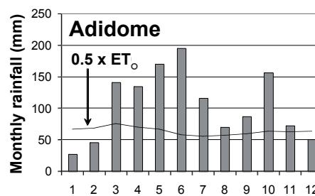
Figure 2.1: Rainfall distribution for the 1990-2000 period.  $ET_o$  is the reference evapotranspiration. Data from CRU, using the HARGREAVES (1994) method for  $ET_o$  calculation.
