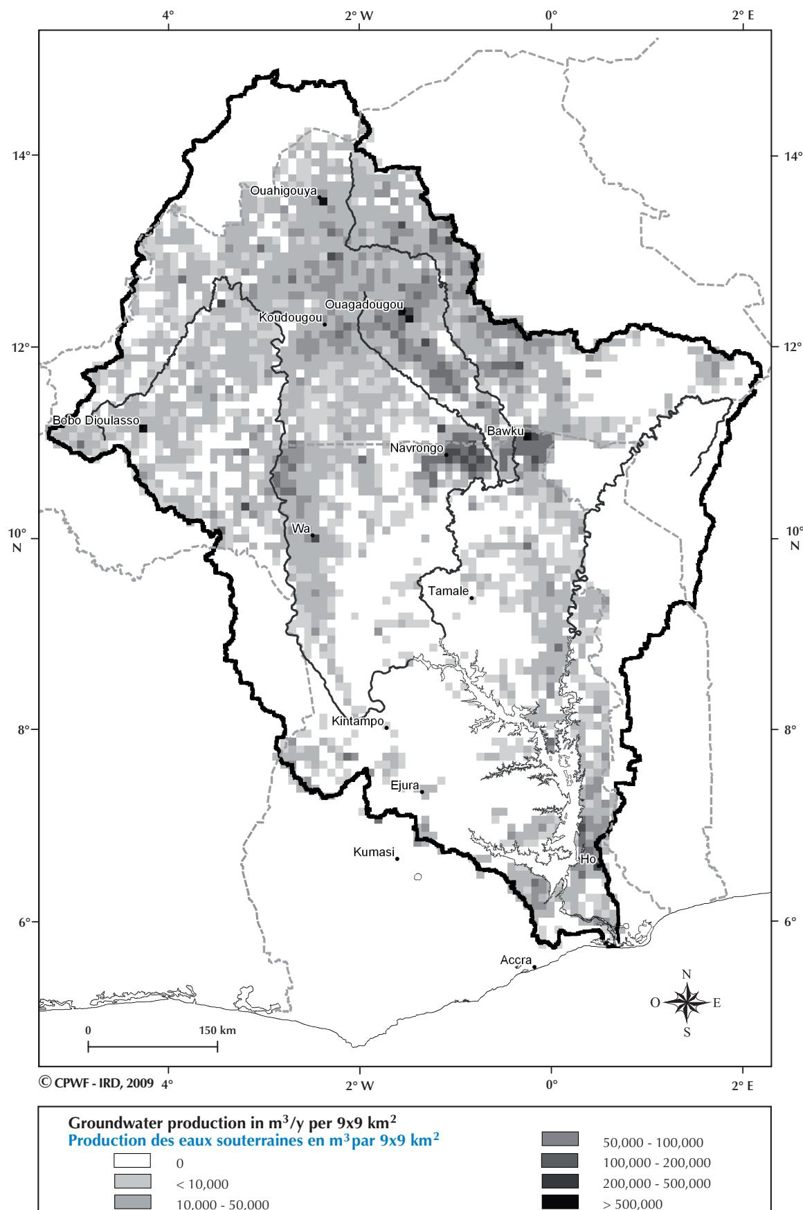
*Spatial distribution of groundwater abstraction in the Ghanaian and Burkinabe parts of the Volta Basin. Units are  $m^3/\text{y}$  per  $9 \times 9 \text{ km}^2$ . Reproduced with permission from MARTIN and VAN DE GIESEN (2005).*
