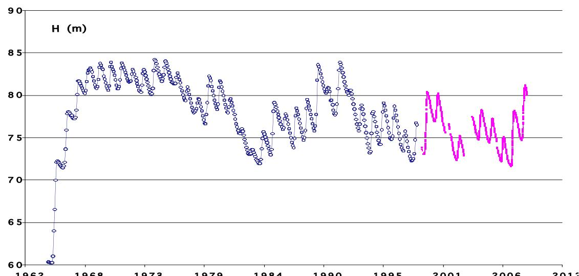
Figure 16.1: The water level in Lake Volta since the closure of the dam. Data from VAN DE GIESEN et al. (2001) and VRA (2009).
