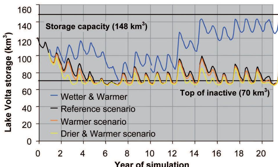
Figure 17.1: Simulation of the water stored in Lake Volta in three scenarios of climate change.
